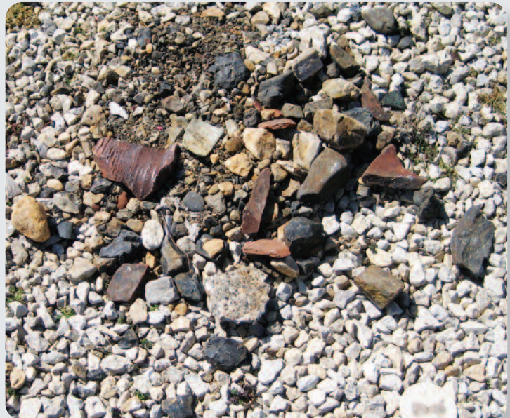
Pieces of clay tile and large debris washed to the headworks during heavy rains.
